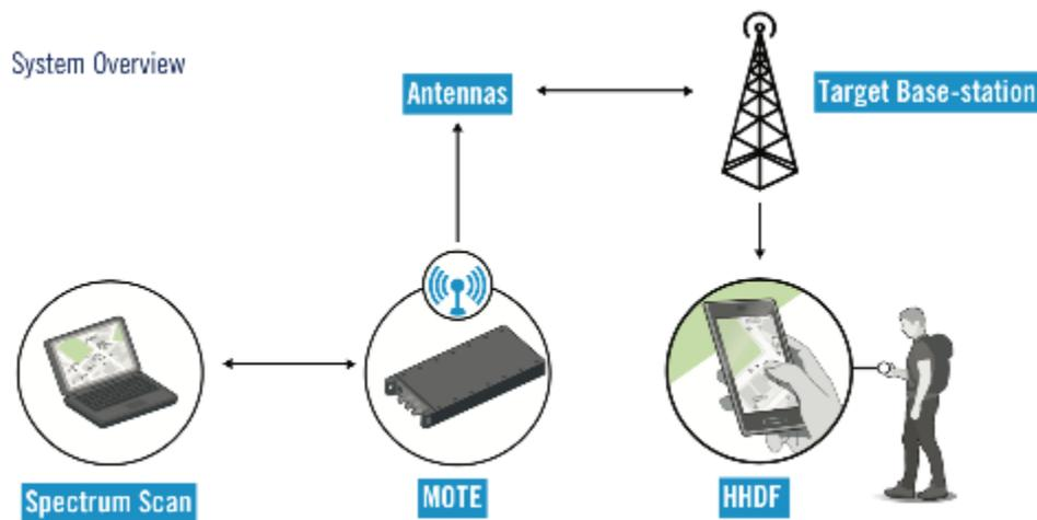
Once more, when a suspicious BTS is detected the user can utilise PEGASUS DF equipment to locate the whereabouts of the system.
